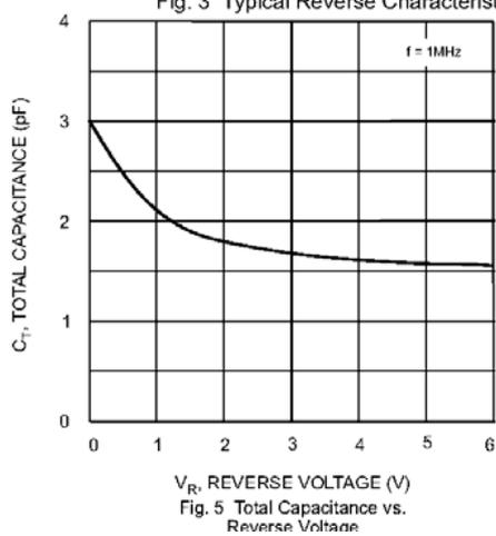
Fig. 5 Total Capacitance vs. Reverse Voltage
